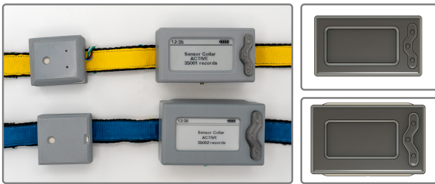
Figure 3: Fully assembled V1 (top) and V2 (bottom) sensor collar systems with CAD illustrations of their respective compute modules shown on the right.
