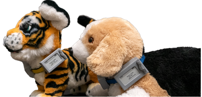
Figure 4: The modular sensor collar worn by Roarin’ Tyler™ & Therabot™
