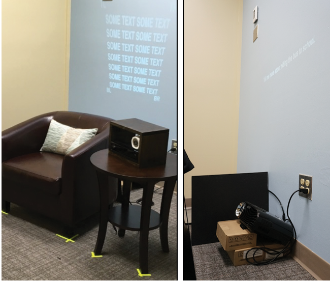
Fig. 5: A low-cost digital projector was combined with an angled mirror to allow the covert projection of text prompts onto the wall behind participants.
