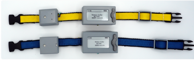
Figure 4: Two versions of the modular sensor collar. Each features a compute module and a basic sensing module.
