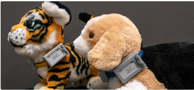
Figure 5: Two zoomorphic robots each wearing a modular sensor collar
